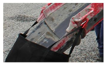
**OPTIONAL -** Carabiners are available by request as an alternate means of securing the Washout Warden to chutes and extenders.
