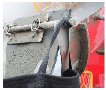
**STEP 2** - Handles can be re-looped over chute pins to obtain a closer fit.
